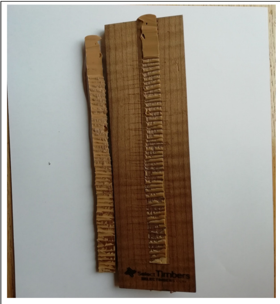
Sikaflex®298: When we pull out from the product it is possible to see that adhesion remain perfect but the wood delaminates when we cut off the bead of the adhesive
