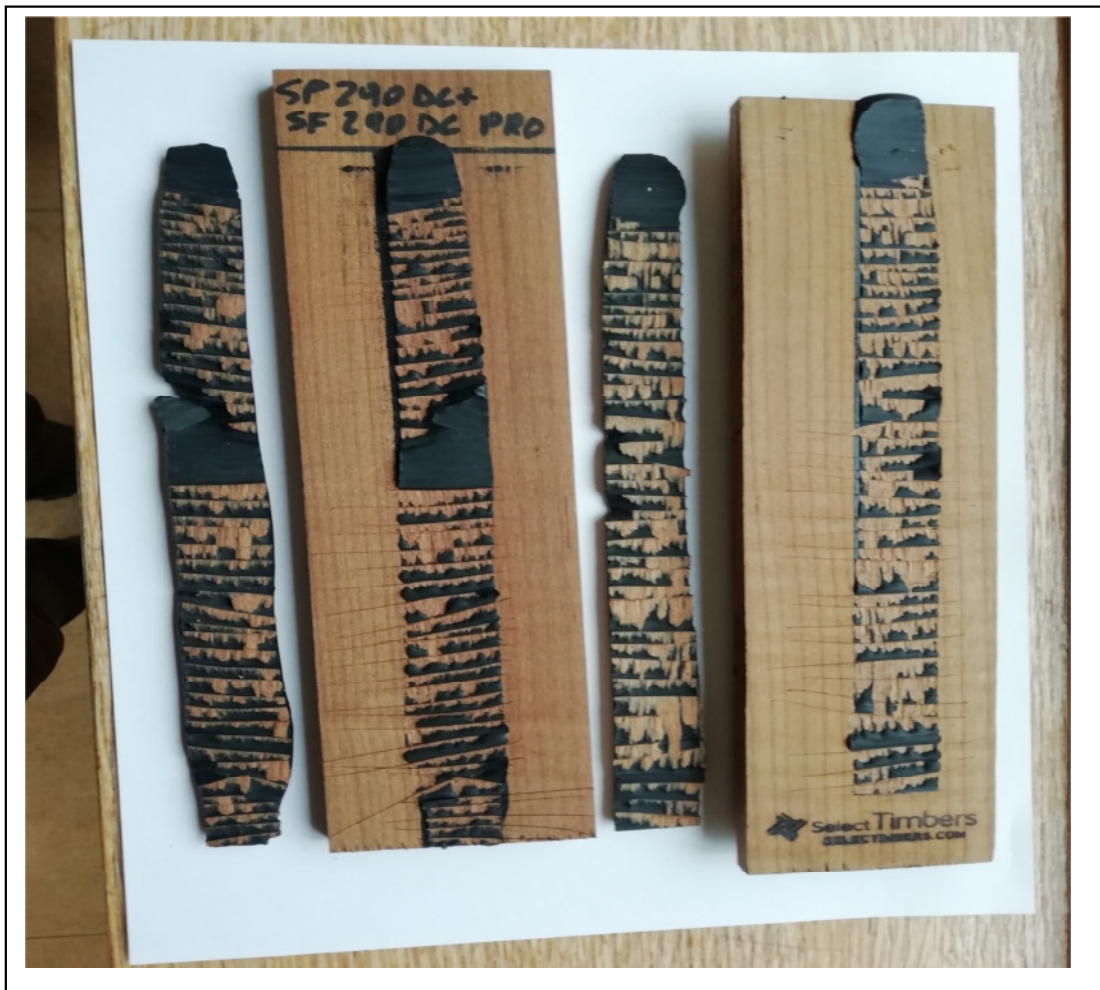
Sikaflex®290 DC PRO: When we pull out from the product it is possible to see that adhesion remain perfect but the wood delaminates when we cut off the bead of the adhesive
