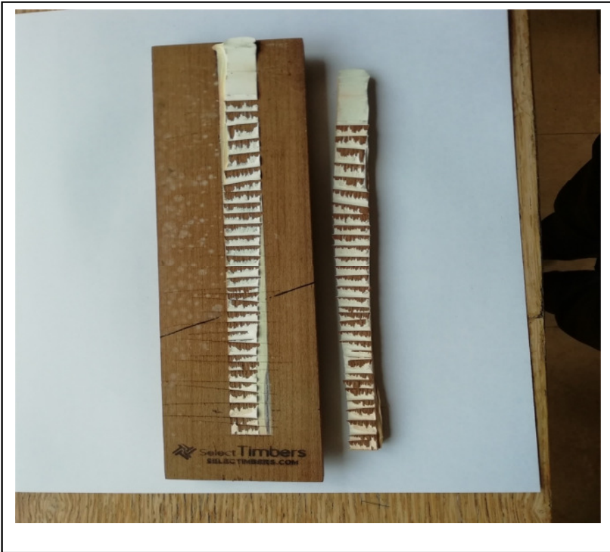
Sikaflex®591: When we pull out from the product it is possible to see that adhesion remain perfect but the wood delaminates when we cut off the bead of the adhesive
